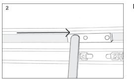
Move the arm into the groove of the window sash.
