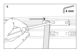
Open the window sash to the maximum opening position required. Finally, tighten the fitting of the arm.
