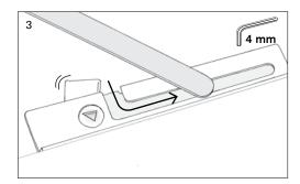
Place the arm into the restrictor fitting and lock the restrictor by turning the screw 90°. Please use VELFAC special Allen key.
