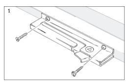
Place the restrictor fitting in the middle of the front edge of the frame. Mark out the drilling holes and pre-drill using a Ø3mm drill. Fasten the restrictor using Ø4 x 50mm screws.
