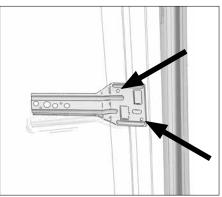
**Securing the lug in the frame.** Slip the taps into the groove and twist into place to secure a good grip. The lug can be turned free again and moved up or down to avoid any positioning issue e.g. a joint between bricks.
