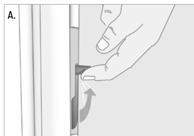
Flush bolt for French Casement mullion and rebated meeting style.
