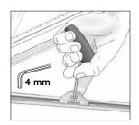
Adjusting the friction brake: Loosen or tighten the screw. Do not oil!
