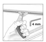
Adjusting the friction brake: Loosen or tighten the screw.
