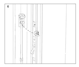
Test before final installation that the eye does not conflict with the window stay when the door / window is closed.
