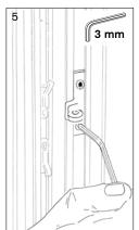
Push the eye of the window stay into the groove of the window sash (4) and fasten it with the top edge approx. 5mm above the window stay (5).
